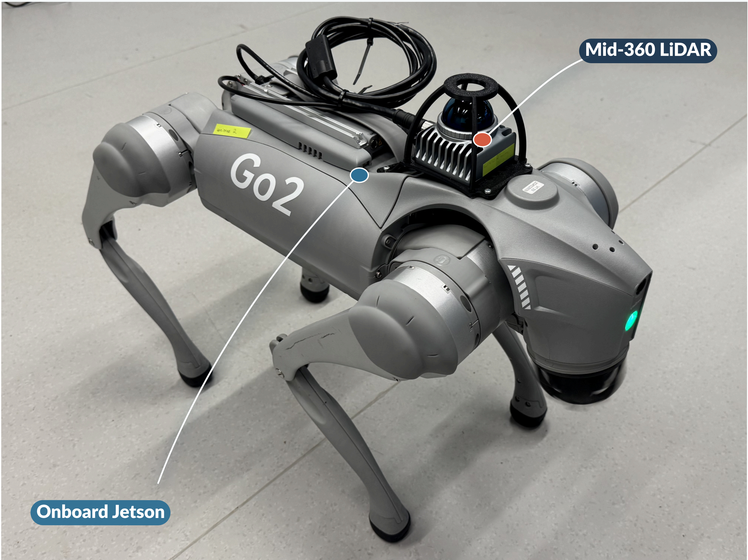
LIVE TEST · LiDAR and tracking ran onboard as a person walked past the stationary robot.
